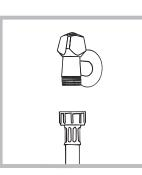
1. Connect the inlet hose by screwing it to a cold water tap using a 3/4 gas threaded connection (see figure).
